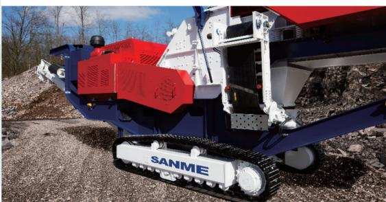
MP-PH Series Mobile Impactor Plant is designed by SK Group Germany, it is an all-purpose, compact and modular impact crushing plant for aggregates and recycling industries.
